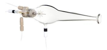
Conventional ICP-MS spray chambers have low transport efficiencies (< 5%) and filter out larger droplets (>5 $\mu$ m) preventing a high percentage of cells from entering the plasma. As most cell lines of interest are larger than 5 $\mu$ m, the spray chamber design for single cell analysis is different from conventional ICP-MS spray chambers.
