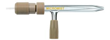
The novel design of the high efficiency nebulizer used in the Glass Expansion HE-SIS system uses a low argon gas flow to provide high nebulization efficiency without rupturing the cell walls.
