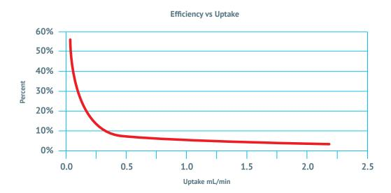
The 50ul/min nebulizer has 50% efficiency and therefore injects 25ul/min into the plasma. On the other hand, the standard 2ml/min nebulizer has 2% efficiency, resulting in 40ul/min of sample injected into the plasma. This means that the MicroMist nebulizer can reduce sample consumption by a factor of 40 and yet the sensitivity is reduced by less than a factor of two.
