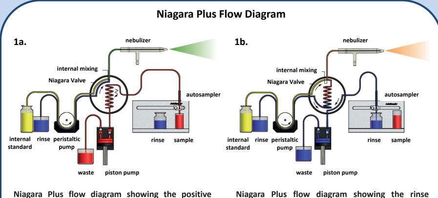
displacement pump rapidly filling the sample loop.
