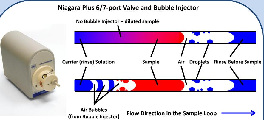
When bubbles are placed between the sample solution and the carrier solution the surface tension restricts the mixing of the sample solution and carrier solution (see bottom tube above). Injecting the bubbles at the end of the sample allows virtually all the sample in the loop to be used for analysis. The bubble injector will put 8-10 bubbles at the end of the sample loop over approximately 25mm of tubing.
